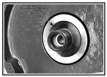
Figure 18. Wheel mounting hub.
